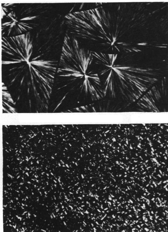
Figure 2 —Micrographs of polypropylene containing 5% of polypropylene oxidation products. In case (a) the polypropylene was dissolved together with oxidation products by heating for 6 h at 125°C; in case (b) the solution of polypropylene in xylene was mixed for 10 min at 125°C with oxidation products. (Crossed polarizers, magnification 80×)
